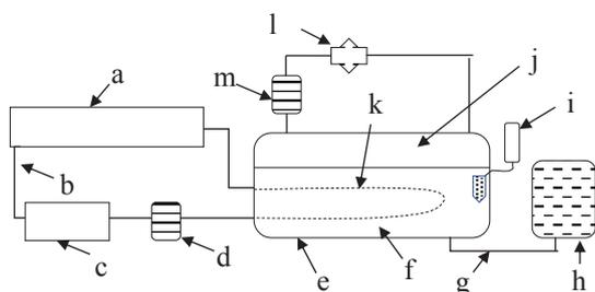
Figure 01. Experimental setup of the soil gas monitoring test. (a) new gas detecting device, (b) gas circulation tube, (c) membrane dryer (d) air pump, (e) soil containing chamber (f) soil, (g) water supplying tube, (h) water container, (i) data logger and soil moisture probe, (j) air in headspace (k) diffusion cell (silicone tube), (l) solenoid valve (m) air pump.
