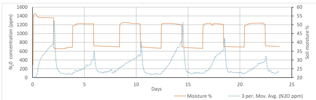
Figure 02. Recorded N<sub>2</sub>O gas concentrations by the new device.
